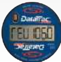
REV Mode shows RPM or RPK unit Programmed for.
