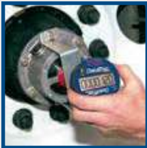
Install DataTrac Pro on wheel end.
